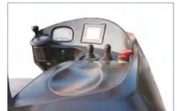
Precise and effortless finger tip control of mast movements and traveling. Comfortable armres and light power steering wheel.
