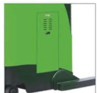
Side battery with roll-out system convenient to replace batteries. The battery upside cover makes you easy to fill the battery.
