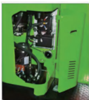
Vertically mounted drive motor with CANbus technology reduces wiring complexity and increases reliability.
