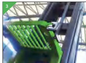
Overhead guard with fans and working light.
