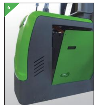
With sideways battery rollers offers quick changes.
