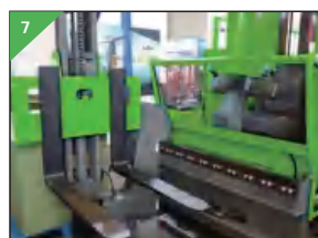
Fork carriage can rotate 180 degrees, flexible for operation in high racking with small aisle.
